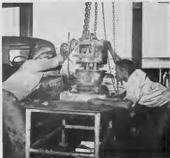
FINISHING TOUCHES on a transmission overhaul requires the combined skills of both A. Hodge, left, and F. Arindell. Lining up the gears is a delicate operation. ULTIMO TOQUE ariba un transmission overhual ta requeri talentanan combiná di A. Hodge, robes, y F. Arindell. Ta un operacion delicada pa line up e gears.
